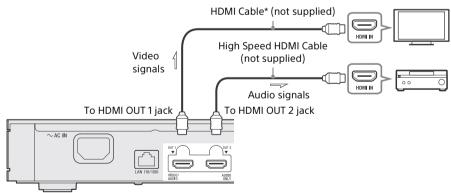
→ If selecting this connection method, set [HDMI Audio Output] in [System settings] to [HDMI2] or [Auto] (page 26).
