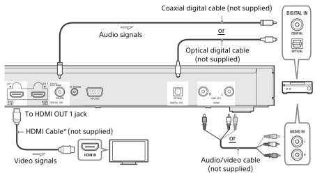
→ If selecting this connection method, set [HDMI Audio Output] in [System settings] to [HDMI1] or [Auto] (page 26).
